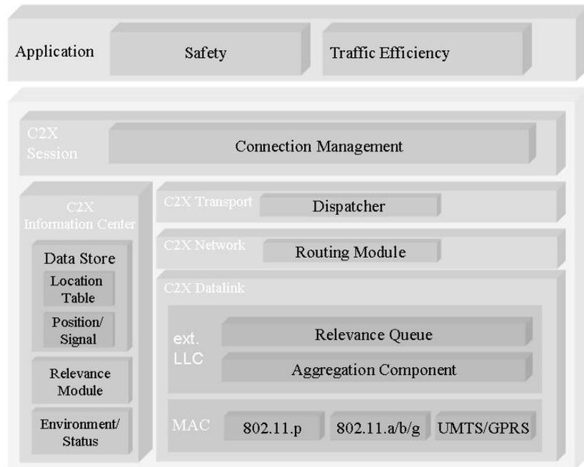
Fig. 2. OpenWAVE Engine Software Architecture
